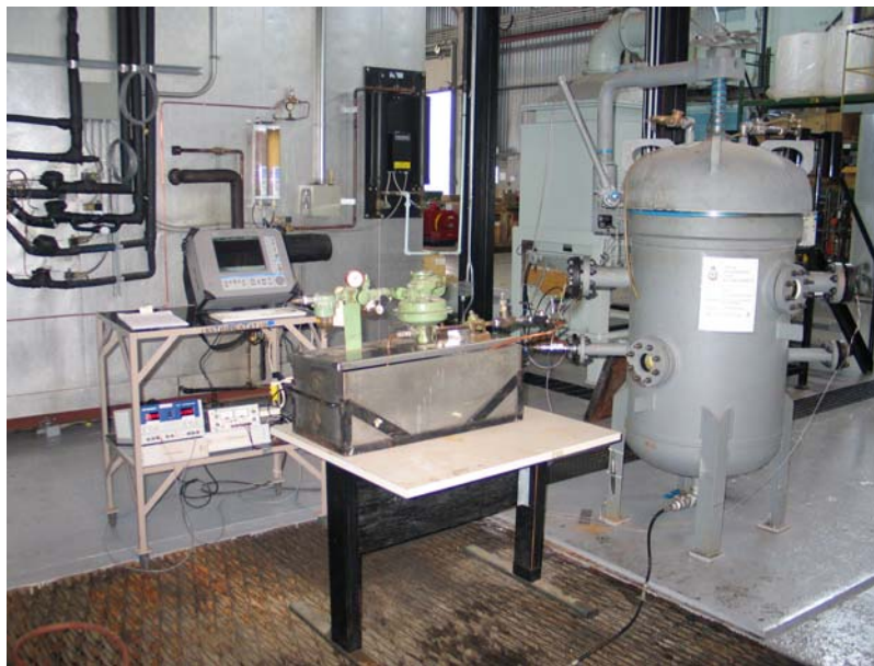
Photograph 2 – Test Set-up for Cyclic Pressure Test
