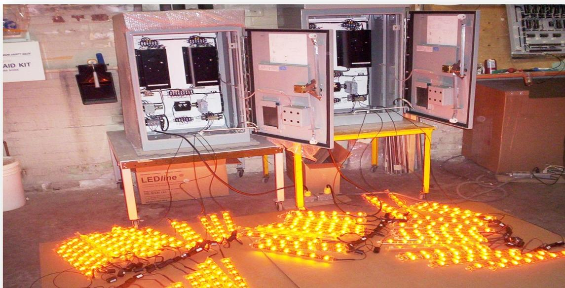
The Master Controller Power Modules, contain custom pulse width Power Modules which takes any power from 90VAC – 220VAC and turns it into the correct low power series circuit voltage, suitable for LEDline® units. There are VDC and other types of power supplies, which vary with application. (Please contact HIL-Tech Ltd. for details).
